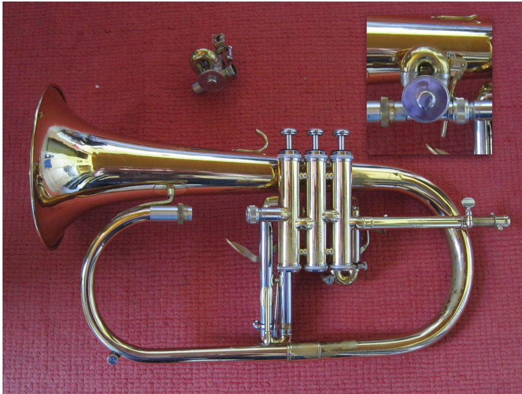
Microtonal Flugelhorn without the fourth rotary valve. Inset: the fourth rotary valve lever mechanism with slider (left) and screw (right) mechanism enabling the exchange of valve.
